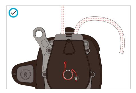
Ensure, especially when descending, that the rope runs untwisted into the Ascender. Twisted ropes caught into the Rope Guide can cause a rope jam and can, in rare cases, result in rope damage.
