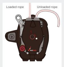
5. Close the Rope Cover and ensure it is locked. The Rope Cover lock should snap into its position. A distinct 'click' should be heard. Never attempt to close the Rope Cover with force.
