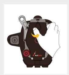
**1**. Open the Rope Cover by pulling on the Rope Cover and pushing the Rope Cover Lock to the right.
