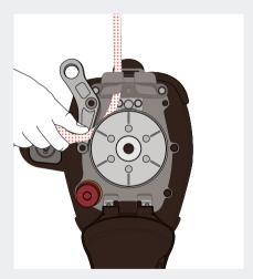
**2.**Feed the rope counter-clockwise through the slot in the Rope Guide and around the Rope Grab.
