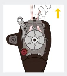
4. Feed the rope through the slot in the Rope Guide. Tighten the rope a little. The rope will be pulled into the Rope Grab and the Rope Cover can be closed more easily.
